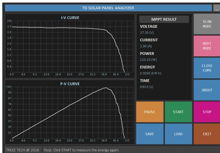
Fig.6 MPPT mode: display voltage, current, power and energy.
